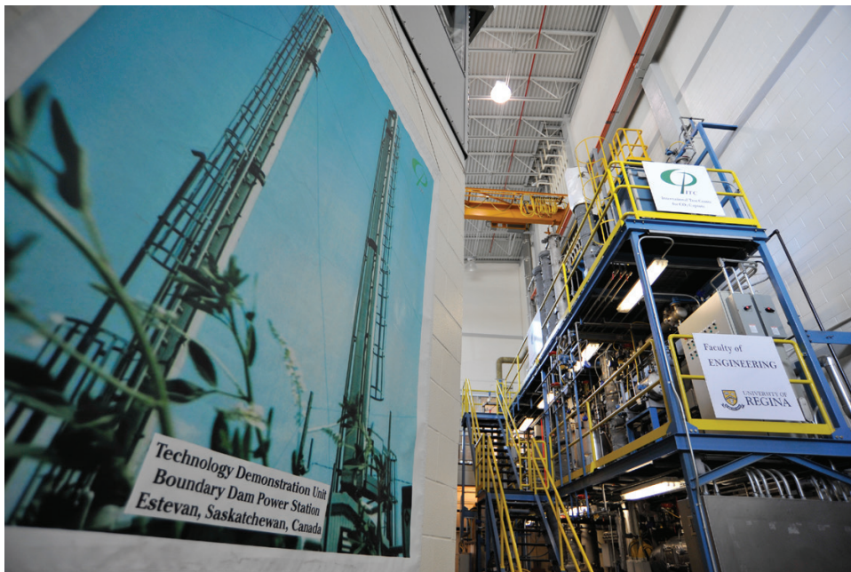
Fig 6: Pre-commercial (indoor) capture demonstration plant (1 ton per day of CO 2 capture) equipped with gas turbine, gas boiler and state-of-the-art monitoring and control systems.
